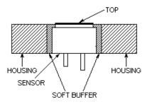
If this part is hold, its characteristics will vary. The top must be free to vibrate.
