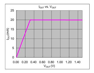
Fig. 3  $I_{OUT}$  vs.  $V_{OUT}$  at  $V_{DD}=5V$
