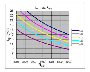
Fig. 4  $I_{OUT}$  vs.  $R_{ext}$  at  $V_{DD}$ = 5V, 4.5V, 4.0V, 3.5V and 3.0V
