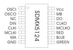
Figure 1 : SDMX5124 Pin Configuration
