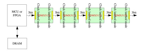
Figure 5: Clock latched mode chain
