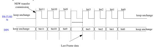
Figure 4: General serial data timing relationship
