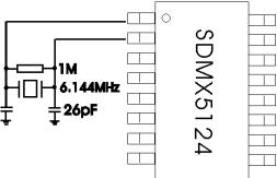
Figure 2: Oscillator configuration
