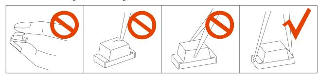
The epoxy resin of encapsulant is fragile, so please avoid scratch or friction over the epoxy resin surface. While handling the product with tweezers, do not hold by the epoxy resin, be careful.
