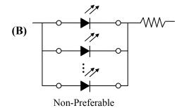
Thermal Design is paramount importance because heat generation may result in the Characteristics decline, such as brightness decreased, Color changed and so on. Please consider the heat generation of the LEDs when making the system design.
