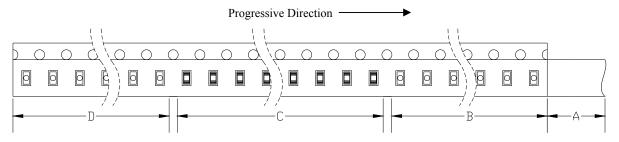
A: Top Cover Tape, 300mm; B: Leader, Empty, 200mm; C: 3000 Lamps Loaded; D: Trailer, Empty, 200mm.
