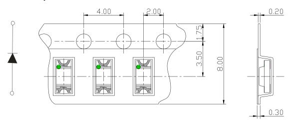
All dimensions in mm, tolerances unless mentioned is  $\pm 0.1$  mm.
