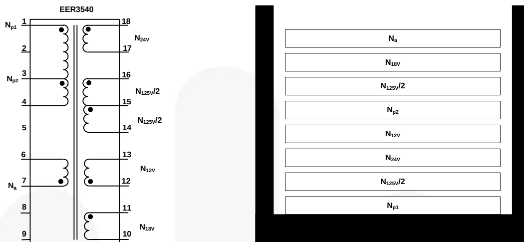
Figure 40. Transformer Schematic Diagram
